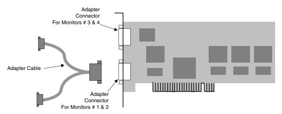
Figure H-1. Compaq/Matrox G200 MMS Quad-Head PCI Graphics Card Layout
